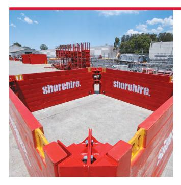
Our Corner Post system is used when a four-sided shoring system is required. With its modular, flexible design, the system can form a wide variety of sizes with varying widths and lengths. The Corner Post System is compatible with our Steel Trench Box range, creating shoring systems from 4m to 6m in size, available for both uppers and lowers.
